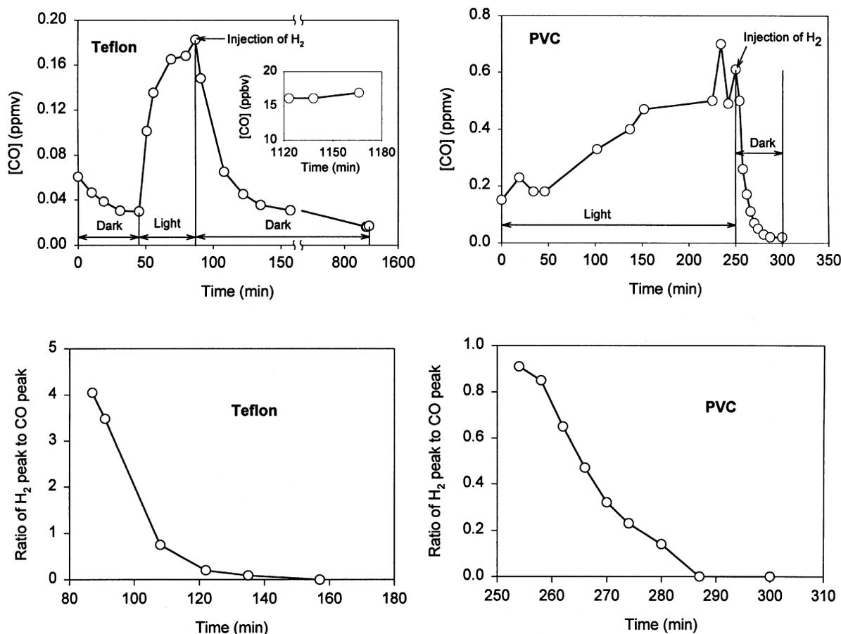
Fig. 6. Upper panels: CO production by plastics (Teflon and PVC) as a function of time under light and dark conditions. Hydrogen spike is used as a dilution tracer. Lower panels: The H<sub>2</sub>/CO peak area ratio as a function of time after the irradiated plastics were darkened. In the Teflon test, the flask had been exposed to sunlight briefly before  $t=0$ . Declining ratios indicate that CO is being evolved continually.
